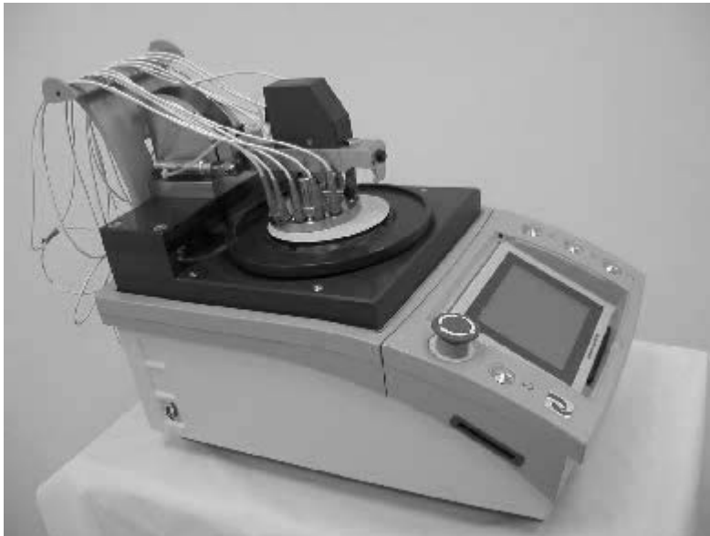
Figure 8.8. Example of a polishing machine that can prepare several fibers simultaneously. (Photo courtesy of Domaille Engineering; www.DomailleEngineering.com .)
