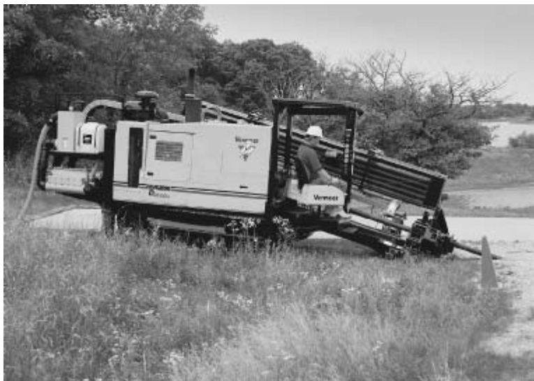
Figure 5.13. Directional boring machine in use. (Photo courtesy of Vermeer Manufacturing Company; www.vermeer.com .)
